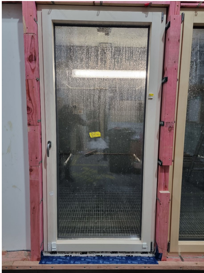
Photo 1: Interior of the Neuffer Eco Plano Wood/Alu Balcony door installed in the test booth.
