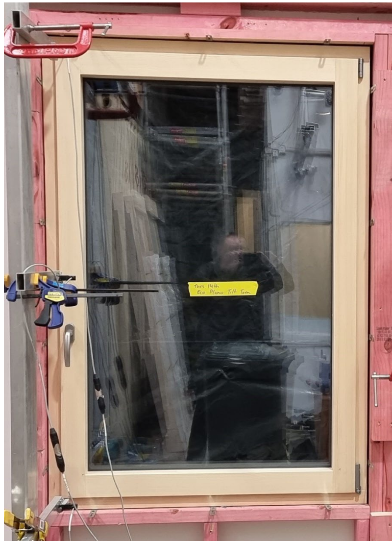
Photo 1: Interior of the Neuffer Eco Plano Wood/Alu Tilt & Turn Sash Window installed in the test booth.
