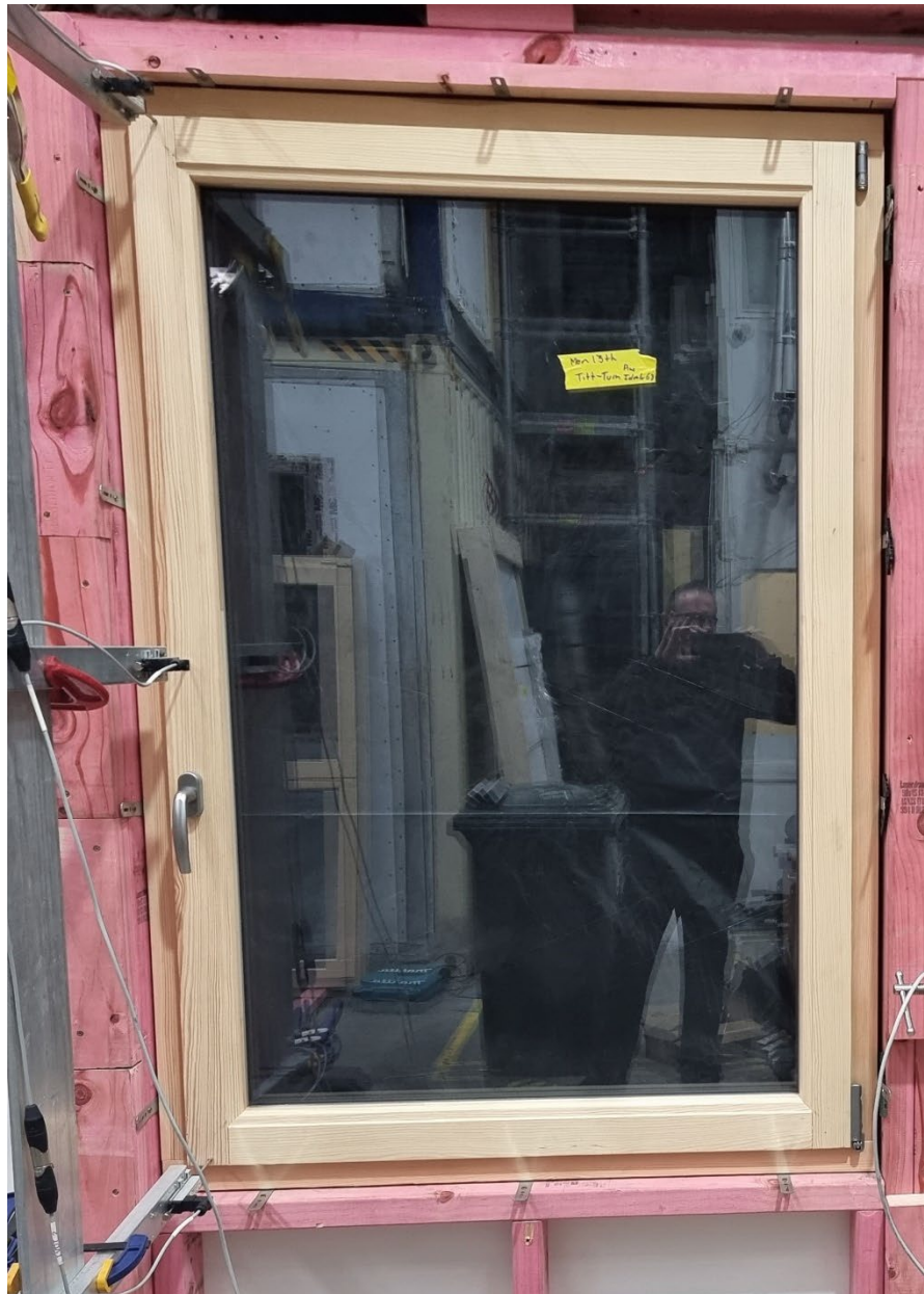
Photo 1: Interior of the Neuffer Idealu 68 Wood/Alu Tilt & Turn Sash Window installed in the test booth.
